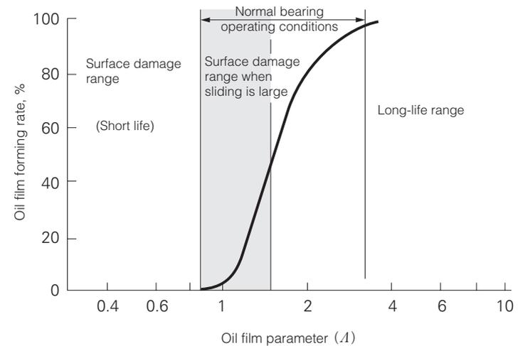
Fig. 2 Effect of oil film on bearing performance
