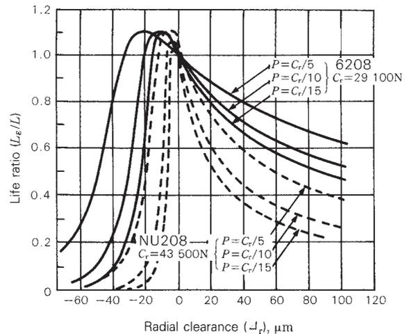
Fig. 2 Radial clearance and bearing life ratio
