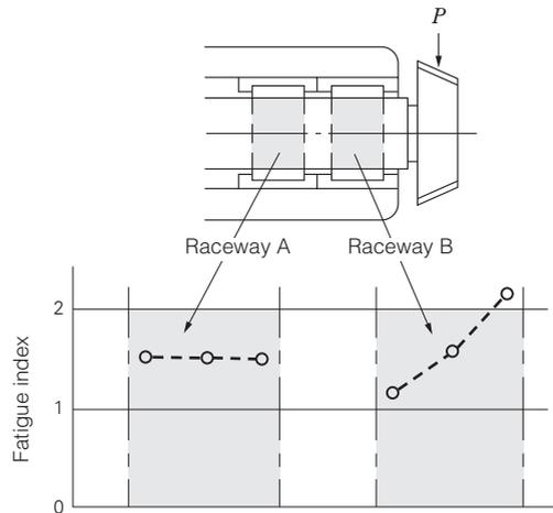
Fig. 7 Distribution of fatigue index in the raceway surface of the pinion shaft
