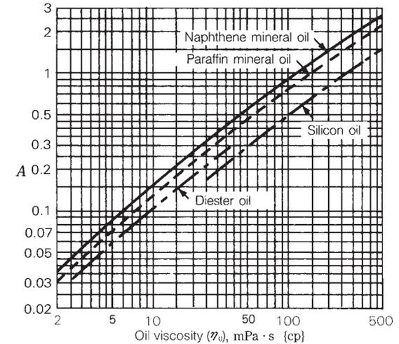
Fig. 4 Term related to lubricant viscosity,  $A$
