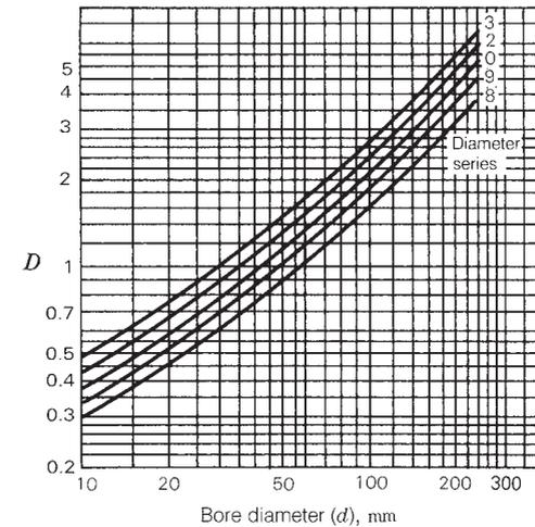
Fig. 5 Term related to bearing specifications,  $D$
