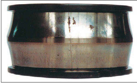
Inner ring fracture
