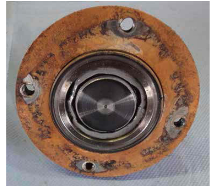
The picture shows that no contamination or rust is present beyond the O-ring.
