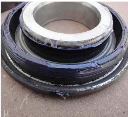
No dirt was able to get through the cassette seal. The seal is in outstanding condition.
