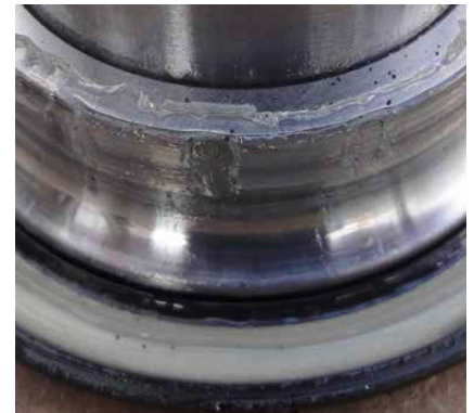
There is no sign of damage or wear to the raceways.
