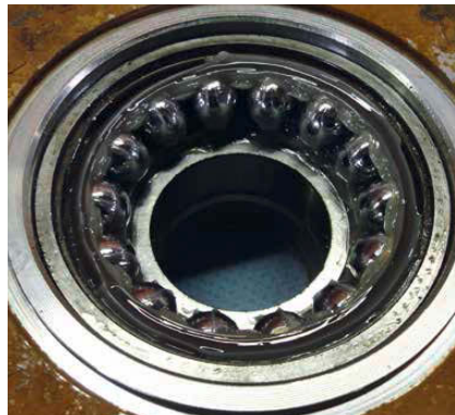
Once the bearing had been dismantled, no dirt was found inside the bearing or in the lubricant.
