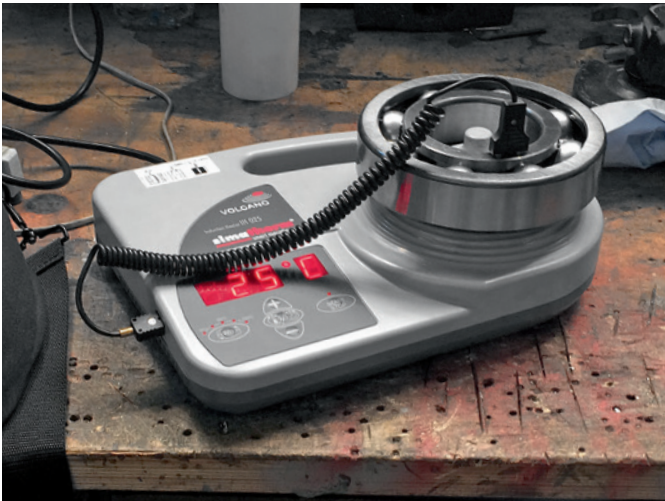
The very portable VOLCANO IH 025 weighs only 3.5 kg but can easily heat parts weighing up to 10 kg to 110°C.
