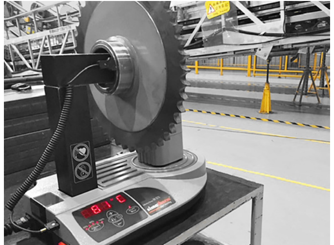
The induction heater IH 070 is the ideal choice for heating the return sprocket for the step chain of an escalator.
