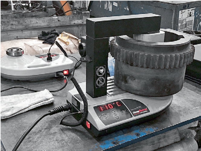
The simatherm induction heaters VOLCANO IH 025 and IH 070 with two differently sized workpieces: the model IH 070 (at the front) heats a gearwheel sleeve to the specified installation temperature.
