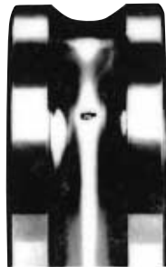
Fig. 5.1 Example of Flaking
