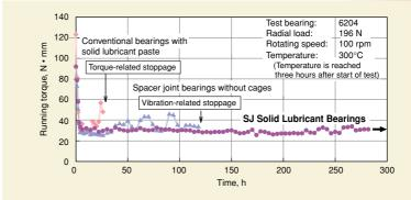
Fig. 1 Durability of bearings in high-temperature normal environments
