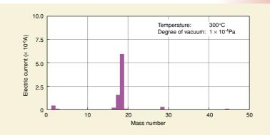
Fig. 3 Analysis results on outgassing of SJ Solid Lubricant Bearings
