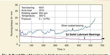
Fig. 2 Durability of bearings in high-temperature vacuum environments
