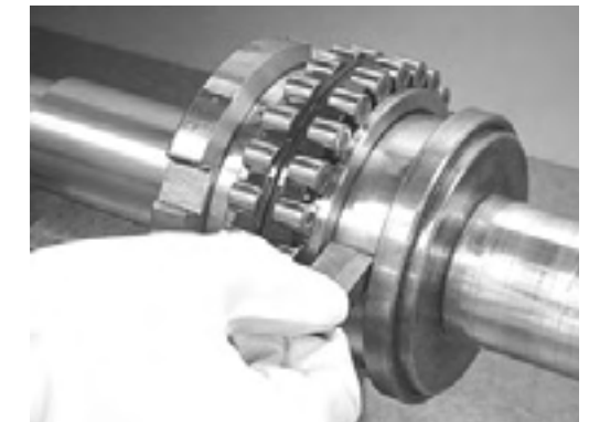
Fig. 1.15 Measurement of Spacer Width
