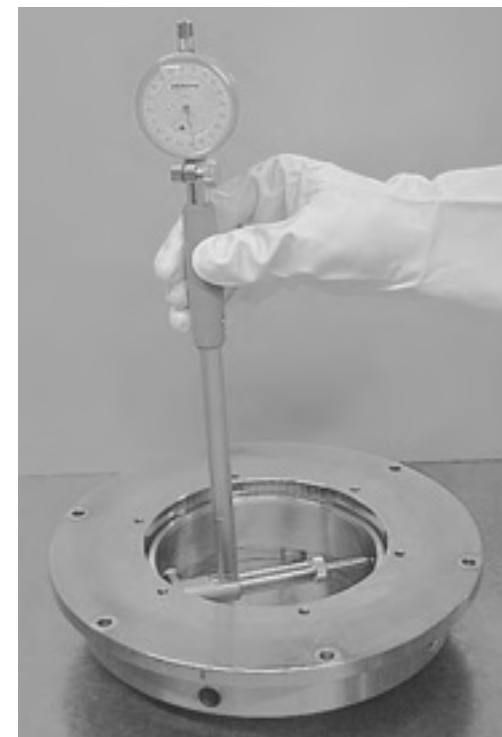
Fig. 1.10 Zero Setting of Cylinder Gauge
