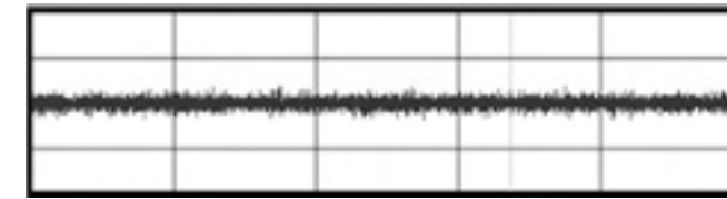
Sound waveform of a normal bearing
