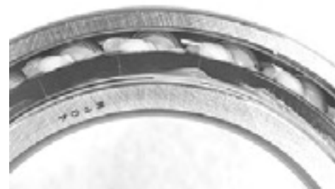
Fig. 1.20 Grease Packed Cylindrical Roller Bearing
