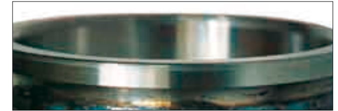
Part: Inner ring of an angular contact ball bearing Symptom: Raceway discoloration; melting occurs at ball pitch intervals Cause: Excessive preload
