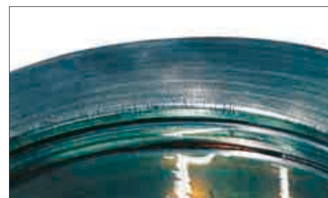
Part: Outer ring of a double-row cylindrical roller bearing Symptom: Thermal cracks occur on the outer ring side face Cause: Abnormal heat generation due to contact sliding between mating part and face of outer ring
