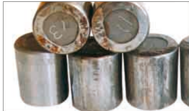
Part: Tapered rollers of a double-row tapered roller bearing Symptom: Stepped wear on the roller end face Cause: Fretting progression due to excessive load while stationary
