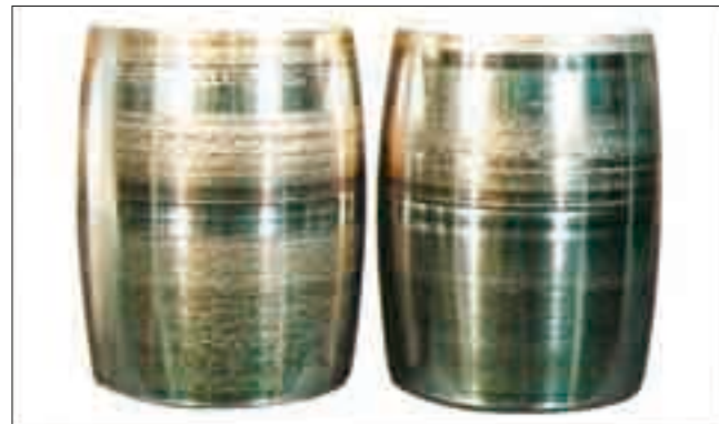
Part: Convex rollers of a spherical roller bearing Symptom: Smearing occurs at the center of the rolling surface Cause: Incorrect lubrication
