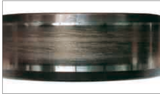
Part: Inner ring of a cylindrical roller bearing Symptom: Smearing occurs circumferentially on raceway surface Cause: Roller slipping due to excessive grease filling
