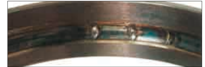
Part: Outer ring of an angular contact ball bearing Symptom: Raceway discoloration; melting occurs at ball pitch intervals Cause: Excessive preload
