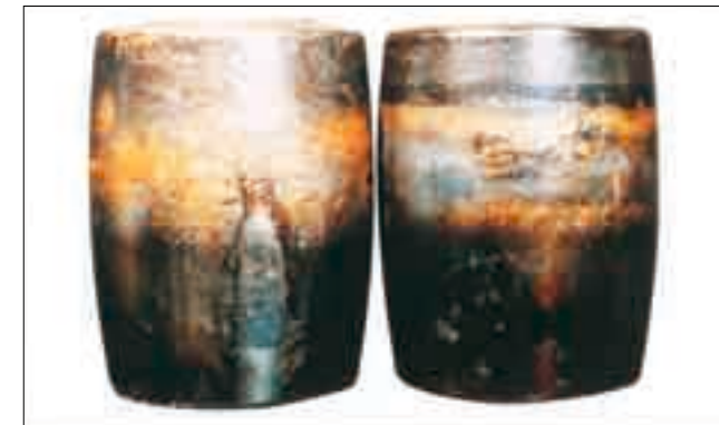
Part: Convex rollers of a spherical roller bearing Symptom: Discoloration and melting of roller rolling surface, adhesion of abrasion fragments from cage Cause: Insufficient lubrication
