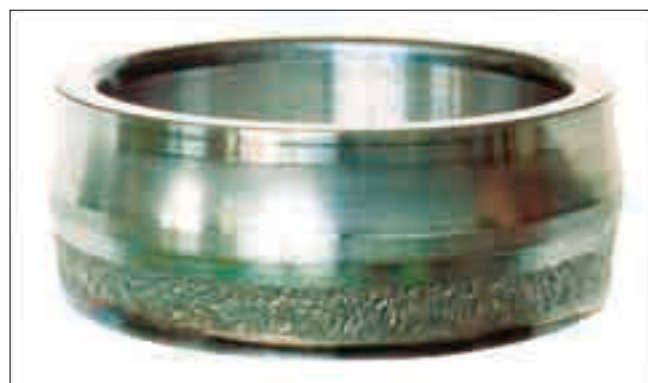
Part: Inner ring of a spherical roller bearing Symptom: Flaking of only one raceway over its entire circumference Cause: Excessive axial load
