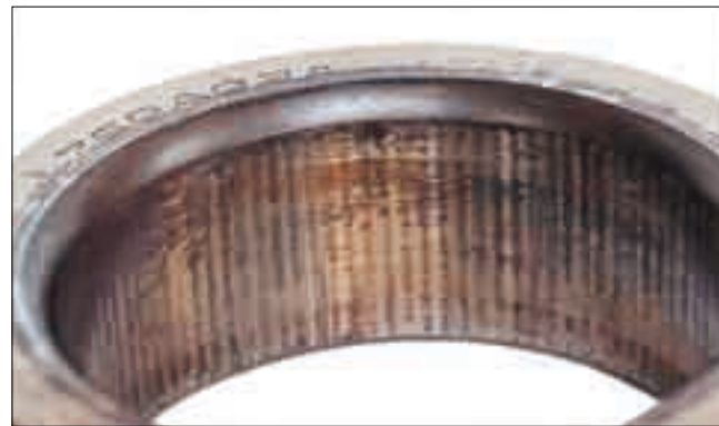
Part: Inner ring of an angular contact ball bearing Symptom: Notable fretting occurs over entire circumference of bore surface Cause: Insufficient interference fit
