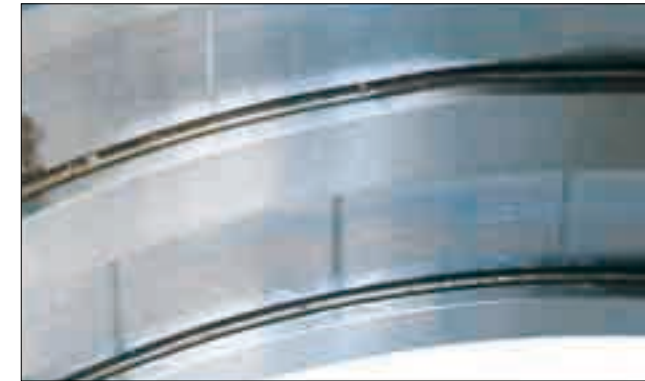
Part: Outer ring of a double-row cylindrical roller bearing Symptom: Fretting occurs on the raceway surface at roller pitch intervals
