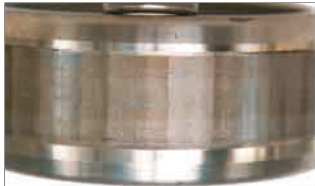
Part: Inner ring of a cylindrical roller bearing Symptom: Many pits occurs due to electrical corrosion; wave-shaped wear on raceway surface Cause: Electrical corrosion
