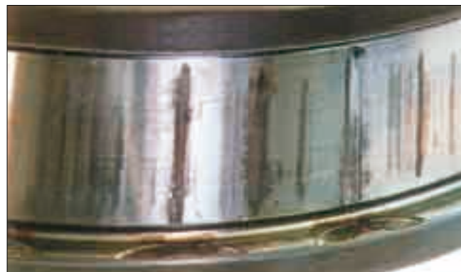
Part: Inner ring of a double-row tapered roller bearing Symptom: Fretting wear of raceway and stepped wear on the rib face Cause: Fretting progression due to excessive load while stationary
