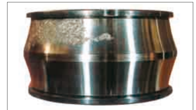
Part: Inner ring of a spherical roller bearing Symptom: Flaking of only one row of raceway Cause: Incorrect lubrication
