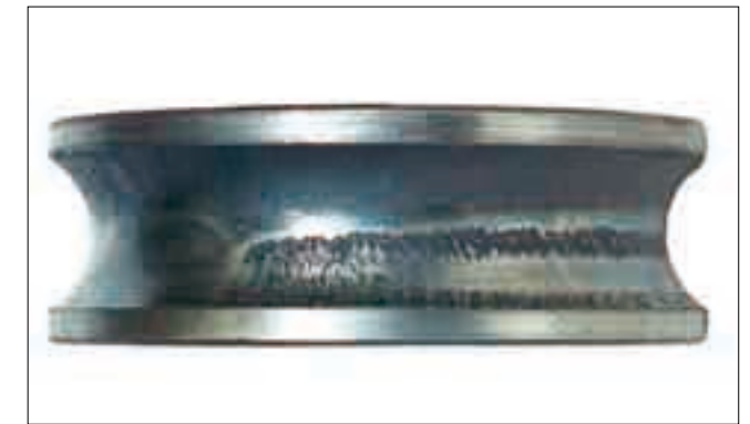
Part: Inner ring of an angular contact ball bearing Symptom: Flaking occurs diagonally along raceway Cause: Improper alignment between shaft and housing during mounting
