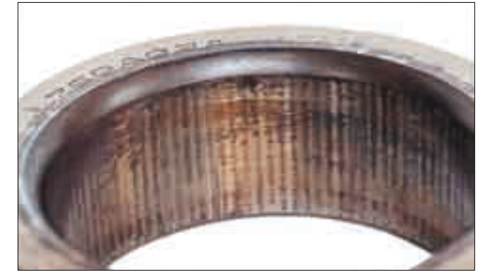
Part: Inner ring of an angular contact ball bearing Symptom: Notable fretting occurs over entire circumference of bore surface Cause: Insufficient interference fit
