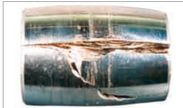
Part: Roller of a spherical roller bearing Symptom: Axial cracks occurs on rolling surface
