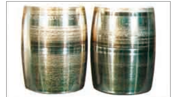
Part: Convex rollers of a spherical roller bearing Symptom: Smearing occurs at the center of the rolling surface Cause: Incorrect lubrication
