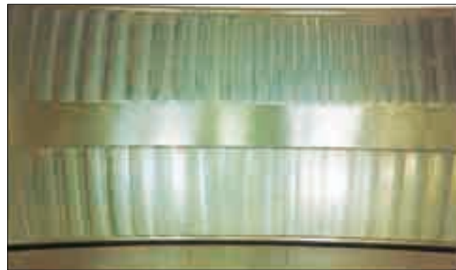
Part: Outer ring of a spherical roller bearing Symptom: Wear having a wavy or concave-and-convex texture on loaded side of raceway surface Cause: Entry of foreign matter under repeated vibration while stationary
