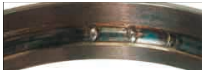
Part: Outer ring of an angular contact ball bearing Symptom: Raceway discoloration; melting occurs at ball pitch intervals Cause: Excessive preload
