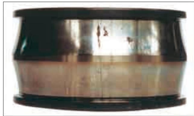
Part: Inner ring of a spherical roller bearing Symptom: Axial cracks occur on raceway surface Cause: Large fitting stress due to temperature difference between shaft and inner ring
