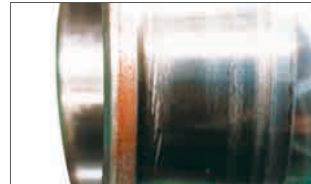
Part: Inner ring of a spherical roller bearing Symptom: Partial smearing occurs circumferentially on raceway surface Cause: Incorrect lubrication
