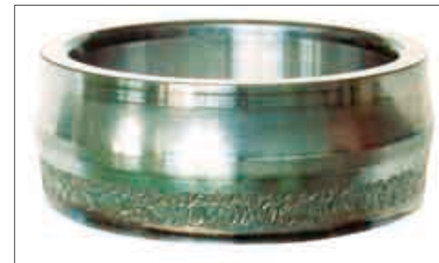
Part: Inner ring of a spherical roller bearing Symptom: Flaking of only one raceway over its entire circumference Cause: Excessive axial load
