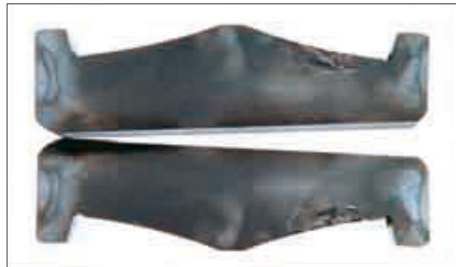
Part: Cross section of a fractured inner ring in a spherical roller bearing Symptom: Origin is directly beneath the raceway surface
