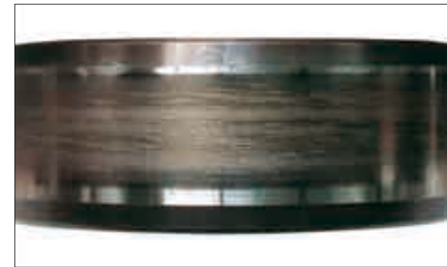
Part: Inner ring of a cylindrical roller bearing Symptom: Smearing occurs circumferentially on raceway surface Cause: Roller slipping due to excessive grease filling
