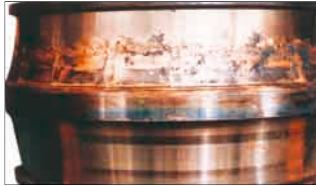
Part: Inner ring of a spherical roller bearing Symptom: Discoloration and melting of raceway; worn particles from the cage were rolled and attached to the raceway Cause: Insufficient lubrication
