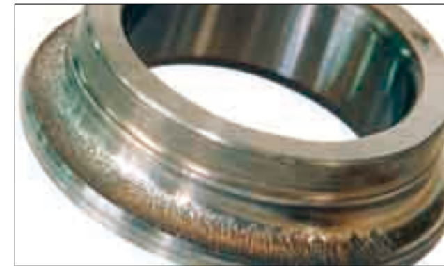
Part: Inner ring of an angular contact ball bearing Symptom: Flaking occurs around half of the circumference of the raceway surface Cause: Incorrect lubrication due to entry of cutting coolant into bearing
