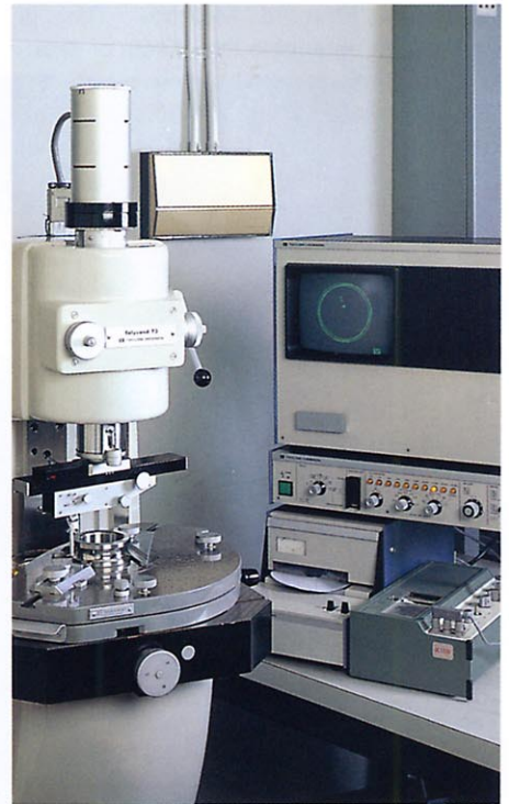
■ High Magnification Out-of-Roundness Measuring Instrument (magnification: 200,000)
