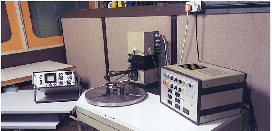
■ Eddy Current Inspection
