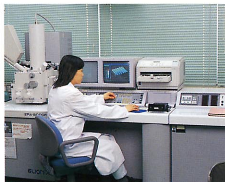
■ Field emission electron probe surface roughness analyzer
