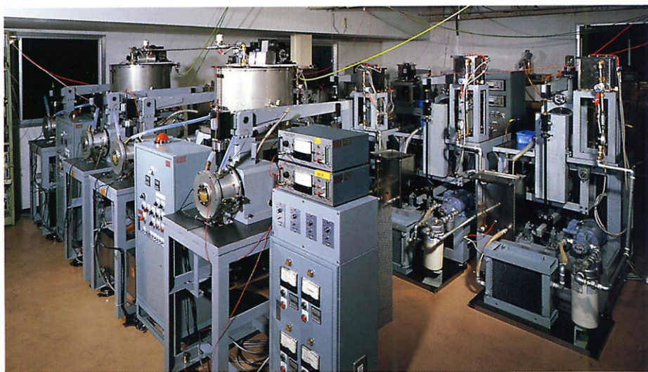
■ Bearing Fatigue Testers
