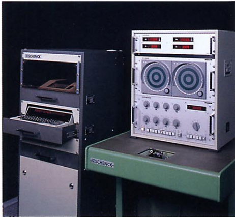
■ Balance Measurement of Roller
