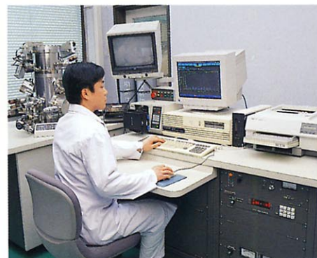
■ Scanning Auger microprobe
