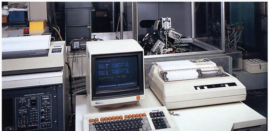
■ X-Ray Metal-Fatigue Test Equipment
