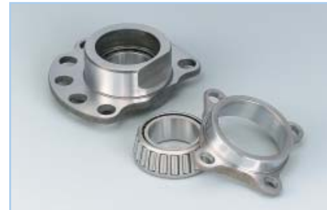
Long Life Tapered Roller Bearings with Outer Mounting Flange The number of parts is reduced by unitization of the housing and outer ring, which also allows for easier assembly.
