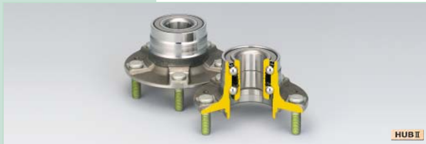
Double-Row Angular Contact Ball Bearings with Outer Mounting Flange (HUB II for Outer Ring Rotation Type) Outer ring rotating hub unit bearing with outer flange for mounting the wheel.
