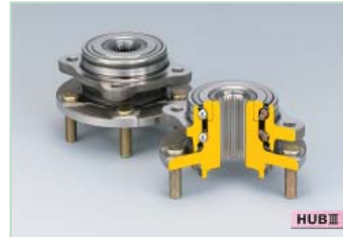
Double-Row Angular Contact Ball Bearings with Inner and Outer Mounting Flange (HUB III for Driven Wheels) Double-row angular contact ball bearing with integral inner and outer mounting flange. Easier mounting because of preset preload.
