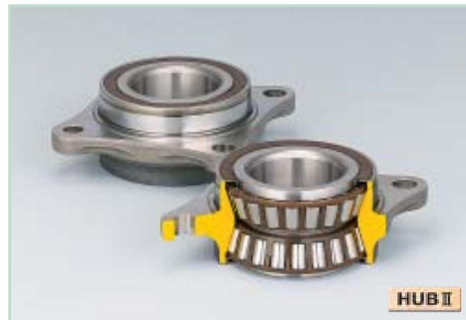
Double-Row Tapered Roller Bearings with Outer Mounting Flange (HUB II for Inner Ring Rotation Type) Inner ring rotating tapered roller hub unit bearing with integral flange for mounting onto knuckle. Suitable for heavy-duty vehicles.
