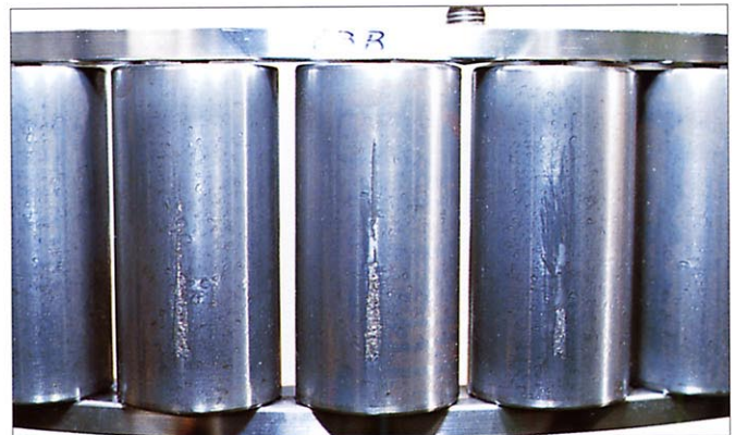
Photo 7-1-10 Part: Rollers of a cylindrical roller bearing Symptom: Premature flaking occurs axially on the rolling surfaces Cause: Scratches caused during improper mounting
