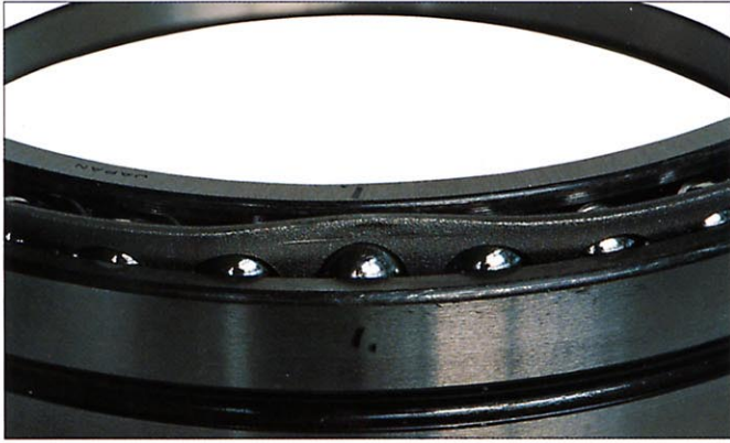
Photo 7-7-5 Part: Cage of an angular contact ball bearing Symptom: Pressed-steel cage deformation Cause: Shock load due to poor handling
