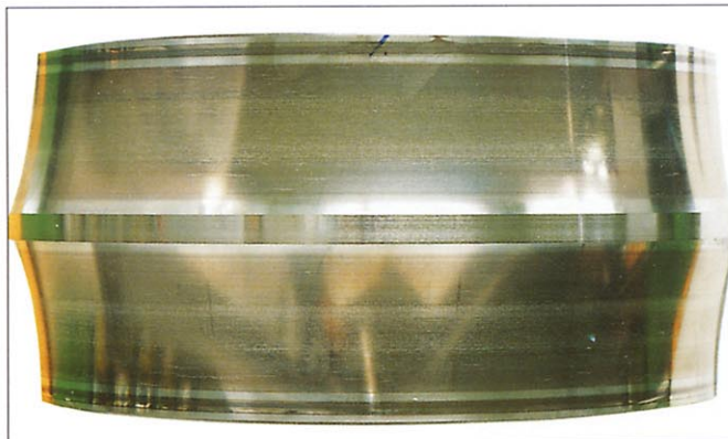
Photo 7-4-3 Part: Inner ring of a spherical roller bearing Symptom: Smearing occurs circumferentially on raceway surface Cause: Poor lubrication
