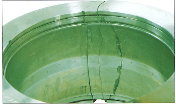
Photo 7-6-5 Part: Raceway surface of outer ring in Photo 7-6-4 Symptom: Outside surface crack developing on the raceway
