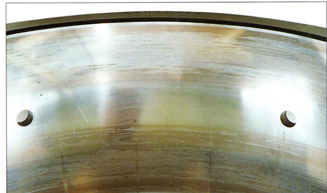
Photo 7-4-4 Part: Outer ring of Photo 7-4-3 Symptom: Smearing occurs circumferentially on raceway surface Cause: Poor lubrication
