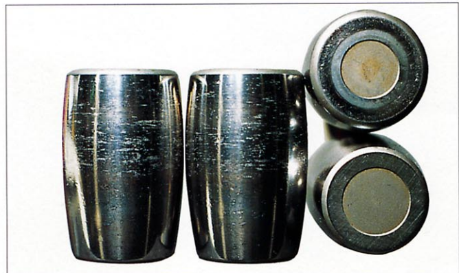
Photo 7-3-2 Part: Convex rollers of Photo 7-3-1 Symptom: Scoring on roller end face Cause: Roller slipping due to sudden acceleration and deceleration
