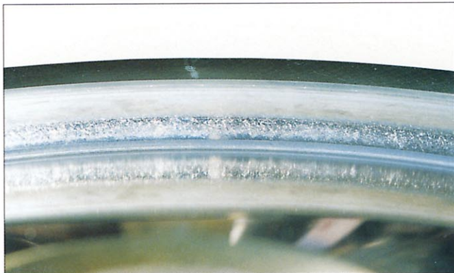
Photo 7-3-3 Part: Inner ring of a tapered roller thrust bearing Symptom: Scoring on the face of inner ring rib Cause: Worn particles become mixed with lubricant, and breakdown of oil film occurs due to excessive load
