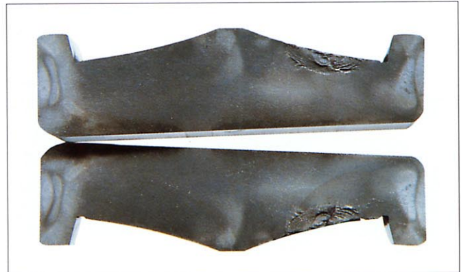
Photo 7-6-7 Part: Cross section of a fractured inner ring in Photo 7-6-6 Symptom: Origin is directly beneath the raceway surface
