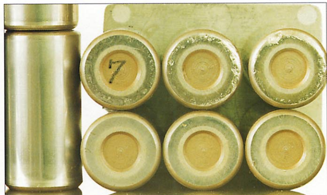
Photo 7-3-4 Part: Rollers of a double-row cylindrical roller bearing Symptom: Scoring on the roller end face Cause: Poor lubrication and excessive axial load
