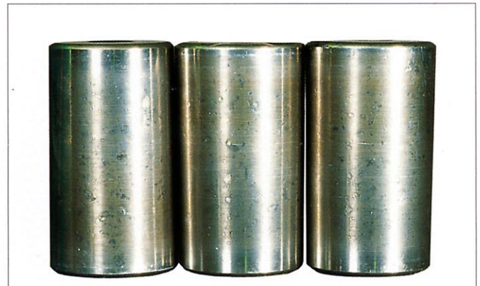
Photo 7-8-4 Part: Tapered rollers of Photo 7-8-3 Symptom: Small and large indentations occur over the rolling surface Cause: Debris caught in the surface
