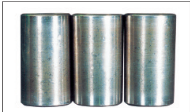
Photo 7-8-4: Part: Tapered rollers of Photo 7-8-3 Symptom: Small and large indentations occur over the rolling surface Cause: Debris caught in the surface
