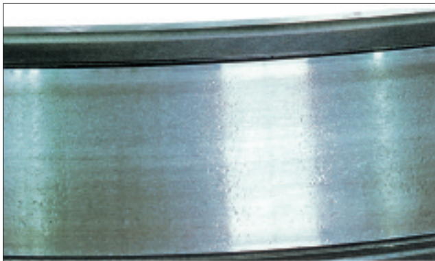
Photo 7-8-3 Part: Inner ring of a tapered roller bearing Symptom: Small and large indentations occur over entire raceway surface Cause: Debris caught in the surface
