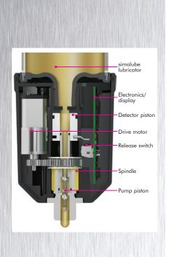
The simalube® IMPULSE ensures reliable lubrication in situations with high counterpressure and long lubrication lines. With the automatic simalube lubricators, this pressure booster pumps greases and oils at up to 10 bar and 0.5 ml per impulse to the targeted lubrication point. The LED display of the intelligent pressure booster provides information continously about the current operating condition, and flashes green when the device is functioning correctly.
