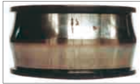
Inner ring fracture
