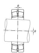
Fig. 3.4 Permissible Misalignment of Spherical Roller Bearings
