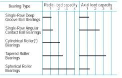
Note(1) The bearings with ribs can take some axial loads.
