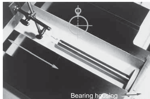
Photo 14.2 Centering of the housing of support bearing
