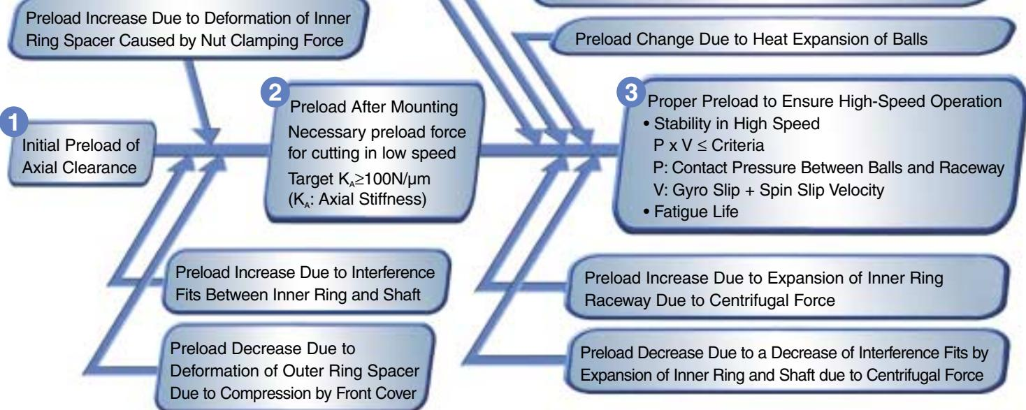
(¹) CAUTION: Preload means the preload values after the bearing has been mounted on the spindle. These after mounted pre-load values will change as a result of the shaft fit requirement of high speed operation and spacer deformation due to nut clamping force. In such case, particularly in high speed applications, it is necessary to adjust the spacer lengths relative to each other in order to compensate for the changes in preload after bearing mounting. Consult NSK for guidance.
