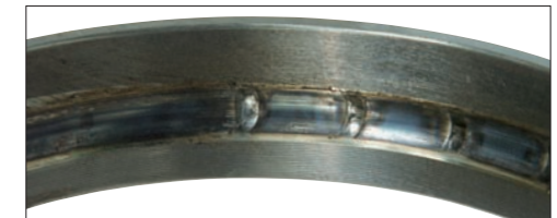
Photo 13-4 Part: Outer ring in Photo 13-3 Symptom: Raceway discoloration, melting at ball pitch intervals Cause: Excessive preload
