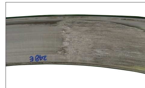
Photo 4-9 Part: Outer ring of a large tapered roller bearing Symptom: Smearing on outer ring raceway surface Cause: High speed, light load, and poor lubrication
