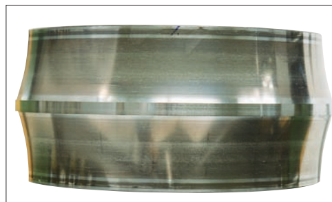
Photo 4-3 Part: Inner ring of a spherical roller bearing Symptom: Smearing circumferentially on raceway surface Cause: Poor lubrication
