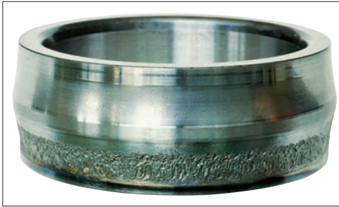
Photo 1-5 Part: Inner ring of a spherical roller bearing Symptom: Flaking of only one raceway over its entire circumference Cause: Excessive axial load
