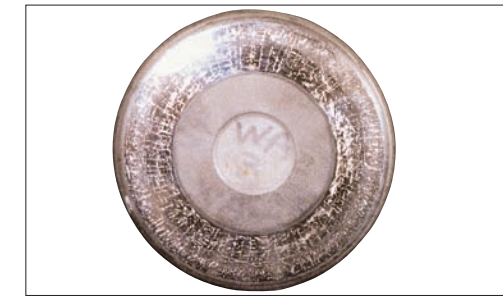
Photo 6-2 Part: Roller of a tapered roller thrust bearing Symptom: Thermal cracks at large end face of roller Cause: Heat generation due to sliding with the inner ring rib under poor lubrication
