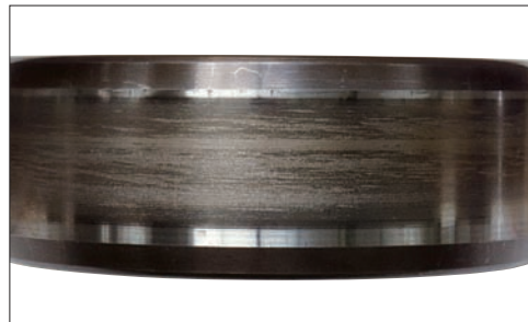
Photo 4-1 Part: Inner ring of a cylindrical roller bearing Symptom: Smearing circumferentially on raceway surface Cause: Roller slippage due to excessive grease filling
