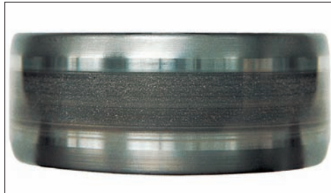
Photo 15-3 Part: Inner ring of a cylindrical roller bearing Symptom: Belt pattern of electrical erosion accompanied by pits on the raceway surface
