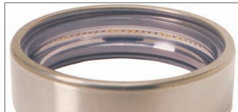
Photo 15-6 Part: Outer ring of a deep groove ball bearing Symptom: Fluting on the raceway surface (high frequency)
