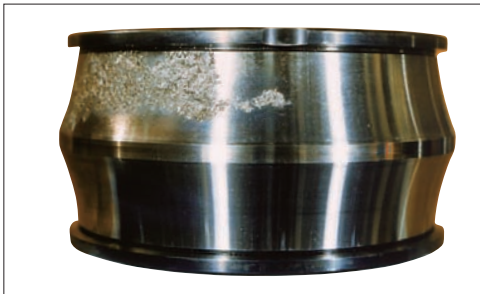
Photo 1-7 Part: Inner ring of a spherical roller bearing Symptom: Flaking of only one raceway Cause: Poor lubrication
