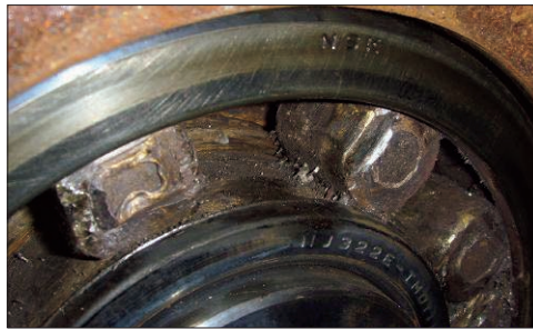
Photo 13-7 Part: Cylindrical roller bearing Symptom: Seizure of roller at ring raceway surface Cause: Excessively small internal clearance generated heat from motion of the inner ring and rollers under high speed and light load
