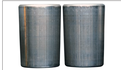
Photo 15-2 Part: Tapered rollers in Photo 15-1 Symptom: Striped pattern of erosion on the rolling surface
