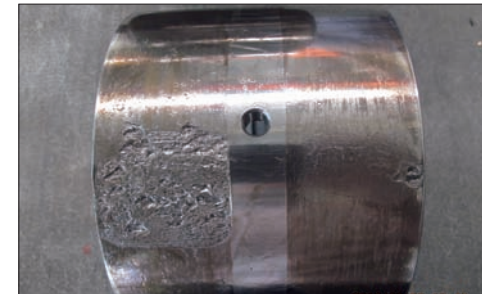
Photo 1-13 Part: Inner ring of a cylindrical roller bearing for Sendzimir mills Symptom: Flaking of the raceway surface Cause: Severe operating conditions and low-viscosity oil lubrication
