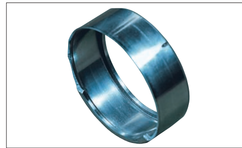
Photo 5-4 Part: Outer ring of a solid type needle roller bearing Symptom: Fracture at the outer ring rib Cause: Roller inclination due to excessive loading (needle rollers are long compared to their diameter; under excessive or uneven loading, rollers become inclined and push against the ribs)
