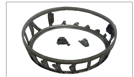
Photo 7-4 Part: Cage of a tapered roller bearing Symptom: Pillar fractures of pressed-steel cage
