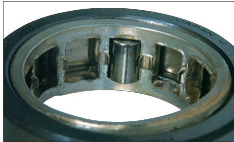
Photo 7-7 Part: Cage of a cylindrical roller bearing Symptom: Deformation and wear of a machined high-tension-brass cage
