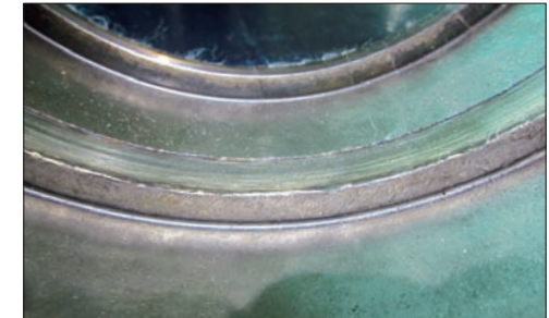
Photo 3-8 Part: Outer ring of a double-row cylindrical roller bearing Symptom: Notable scoring on the face of an outer ring rib Cause: Excessive axial load
