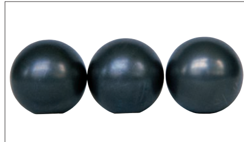
Photo 15-4 Part: Balls of a deep groove ball bearing Symptom: A dark color covering the entire ball surface
