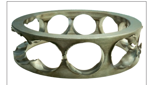
Photo 7-2 Part: Cage of an angular contact ball bearing Symptom: Pocket pillar fractures from a cast-iron machined cage Cause: Abnormal load action on cage due to misaligned mounting between inner and outer rings
