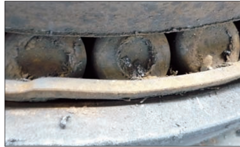
Photo 13-6 Part: Rollers of a large tapered roller bearing Symptom: Seizure at large end face of roller Cause: Poor lubrication and excessive axial load
