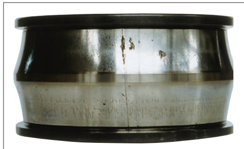
Photo 6-6 Part: Inner ring of a spherical roller bearing Symptom: Axial cracks on raceway surface Cause: Large fitting stress due to temperature difference between shaft and inner ring
