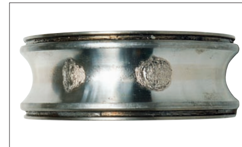
Photo 1-15 Part: Inner ring of deep groove ball bearing Symptom: Flaking of raceway at ball pitch Cause: Dents due to shock load during mounting
