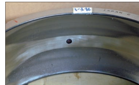
Photo 10-3 Part: Outer ring of a spherical roller bearing Symptom: Wear on loaded side of raceway surface Cause: Low speed, heavy load, and poor lubrication (no oil film)
