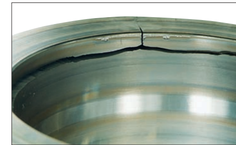
Photo 6-3 Part: Outer ring of a double-row cylindrical roller bearing Symptom: Cracks propagated outward in the axial and circumferential directions from the flaking origin on the raceway surface Cause: Flaking from a flaw due to shock load
