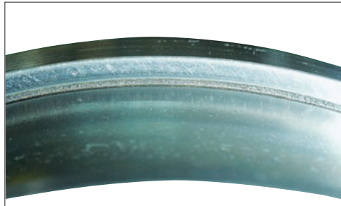
Photo 3-1 Part: Inner ring of a spherical roller bearing Symptom: Scoring on large rib face of inner ring Cause: Roller slippage due to sudden acceleration and deceleration
