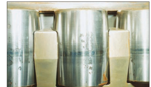
Photo 16-4 Part: Rollers of a spherical roller bearing Symptom: Pit-shaped rust on rolling contact surface, corroded portions Cause: Condensation during storage
