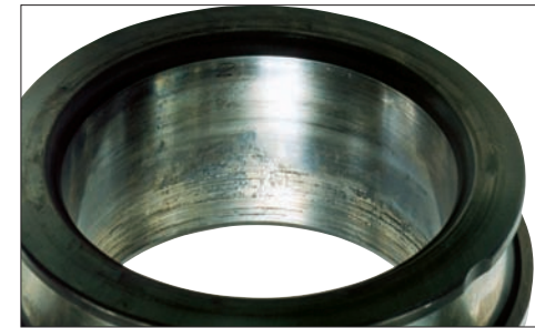
Photo 14-1 Part: Inner ring of a spherical roller bearing Symptom: Creep accompanied by scoring of bore surface Cause: Insufficient interference
