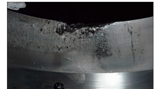
Photo 10-4 Part: Outer ring of a spherical roller bearing (enlargement) Symptom: Combined flaking and wear on the raceway Cause: Insufficient oil film due to poor lubrication led to wear (primary damage) that progressed to flaking (secondary damage)
