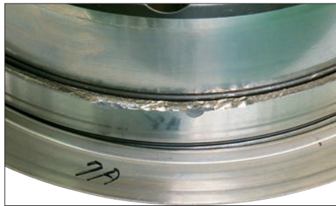
Photo 5-1 Part: Inner ring of a double-row cylindrical roller bearing Symptom: Chipping at the center rib Cause: Excessive load during mounting
