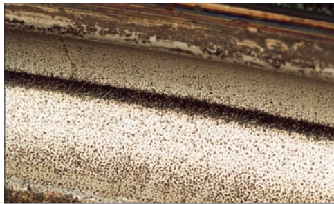
Photo 9-1 Part: Outer ring of a slewing bearing Symptom: Pitting on the raceway surface Cause: Rust at bottom of indentations
