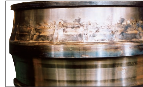
Photo 13-1 Part: Inner ring of a spherical roller bearing Symptom: Discoloration and melting of raceway. Worn particles from the cage rolled off and attached to the raceway. Cause: Insufficient lubrication
