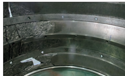
Photo 6-9 Part: Outer ring of four-row tapered roller bearing Symptom: Secondary damage after flaking on outer ring raceway surface
