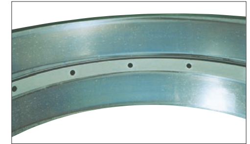
Photo 8-2 Part: Outer ring of a double-row tapered roller bearing Symptom: Indentations on raceway surface Cause: Debris caught in the surface
