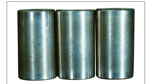
Photo 8-4 Part: Tapered rollers of Photo 8-3 Symptom: Small and large indentations over the rolling surface Cause: Debris caught in the surface
