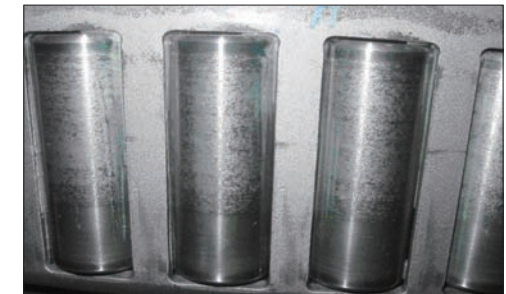
Photo 4-8 Part: Rollers of a large cylindrical roller bearing Symptom: Smearing on rolling surface Cause: Light load and poor lubrication
