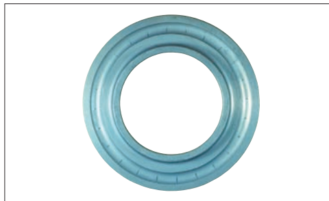
Photo 12-3 Part: Outer ring of a thrust ball bearing Symptom: False brinelling of raceway surface at ball pitch intervals Cause: Repeated vibration with a small oscillating angle
