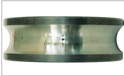
Photo 12-1 Part: Inner ring of a deep groove ball bearing Symptom: False brinelling on the raceway Cause: Vibration from an external source while stationary
