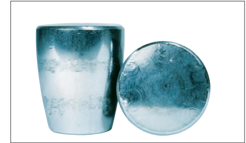
Photo 3-6 Part: Convex rollers of Photo 3-5 Symptom: Scoring on the roller end face Cause: Debris caught in surface and excessive axial load
