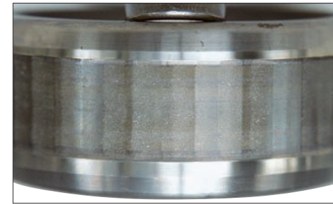
Photo 10-1 Part: Inner ring of a cylindrical roller bearing Symptom: Pits and wave-shaped wear on raceway surface Cause: Electrical erosion
