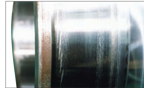
Photo 4-5 Part: Inner ring of a spherical roller bearing Symptom: Partial smearing circumferentially on raceway surface Cause: Poor lubrication
