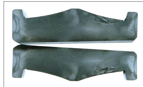
Photo 6-7 Part: Cross section of a fractured inner ring in Photo 6-6 Symptom: Flaking origin directly beneath the raceway surface
