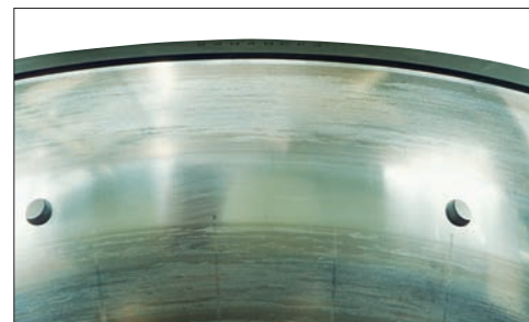
Photo 4-4 Part: Outer ring of Photo 4-3 Symptom: Smearing circumferentially on raceway surface Cause: Poor lubrication
