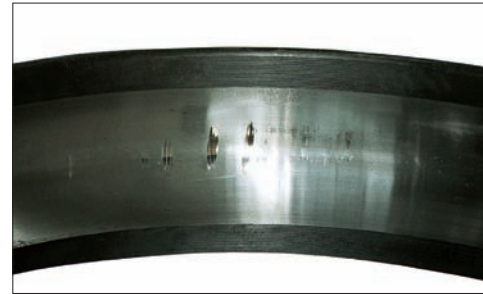
Photo 12-2 Part: Outer ring of Photo 12-1 Symptom: False brinelling on the raceway Cause: Vibration from an external source while stationary
