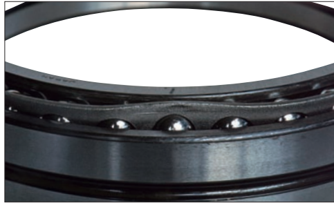
Photo 7-5 Part: Cage of an angular contact ball bearing Symptom: Pressed-steel cage deformation Cause: Shock load due to poor handling
