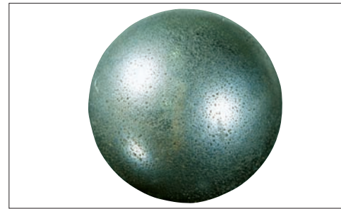
Photo 9-2 Part: Ball of Photo 9-1 Symptom: Pitting on the rolling element surface
