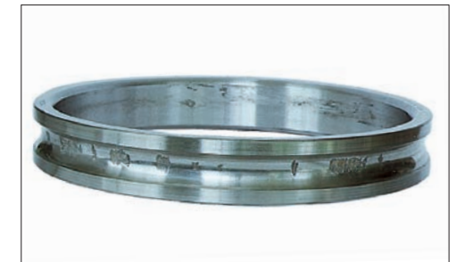
Photo 1-16 Part: Inner ring of an angular contact ball bearing Symptom: Flaking of raceway at ball pitch Cause: Dents due to shock load while stationary
