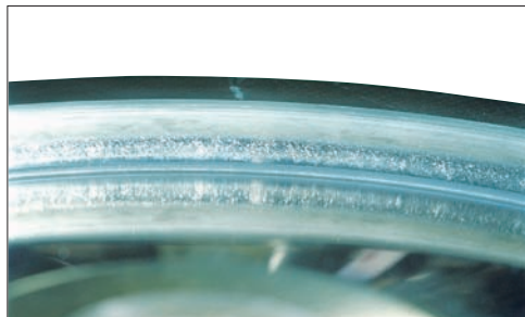
Photo 3-3 Part: Inner ring of a tapered roller thrust bearing Symptom: Scoring on the face of inner ring rib Cause: Worn particles mixed with lubricant and breakdown of oil film due to excessive load
