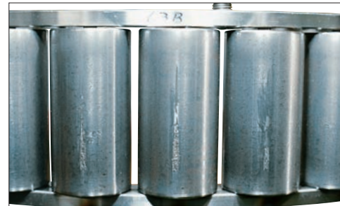
Photo 1-8 Part: Rollers of a cylindrical roller bearing Symptom: Premature flaking of rolling surfaces axially Cause: Scratches caused during improper mounting
