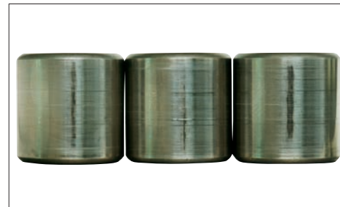
Photo 12-4 Part: Rollers of a cylindrical roller bearing Symptom: False brinelling on rolling surface Cause: Vibration from an external source while stationary
