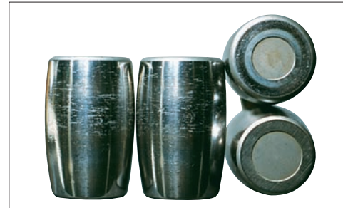
Photo 3-2 Part: Convex rollers of Photo 3-1 Symptom: Scoring on roller end face Cause: Roller slippage due to sudden acceleration and deceleration
