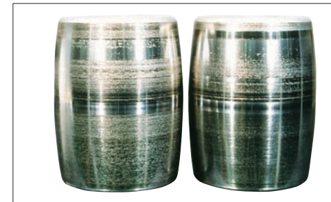
Photo 4-7 Part: Convex rollers of Photo 4-5 Symptom: Smearing at the center of the rolling surface Cause: Poor lubrication
