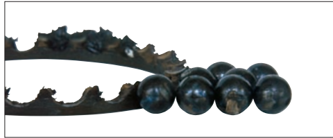
Photo 13-5 Part: Balls and cage of Photo 13-3 Symptom: Cage damaged by melting, balls discolored and melted Cause: Excessive preload
