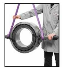
The Bearing Handling Tool is ideally suited for professionally and securely lifting large, heavy bearings. The BHT reduces the risk of accidents and bearing damage. The BHT encloses the outer race of the bearing with a steel band. With two handles on opposite sides and two carrying belts, the bearing can be easily transported with a lifting crane. The bore remains open so the bearings can be easily placed onto a shaft.
