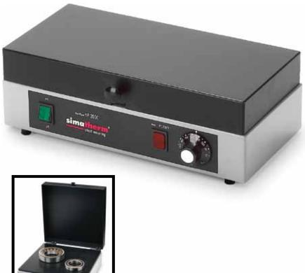
These electric hot plates with thermostatcontrolled bearing heating are especially suited for heating small bearings or small machine parts. The temperature is infinitely adjustable from 50°C to 200°C.
