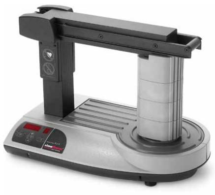
The large simatherm induction heater for roller bearings and other circular metal workpieces up to 600 mm bore diameter and a cross section of 250 x 250 mm. With the integrated time and temperature controls, roller bearings can be heated to the prescribed 110°C while other circular metal workpieces can be heated to 400°C.
